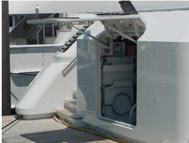
Application: Two 22-38-400 gas springs, 2342 Newton force each with custom made brackets.
